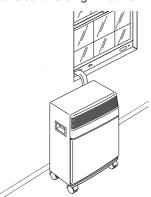
If you have a sliding door, use the additional set provided in order to extend the accessory to the desired length; joining the two parts, adjust the total length according to your needs then, fit the bracket with the relevant nuts, close the door and connect the hose.
